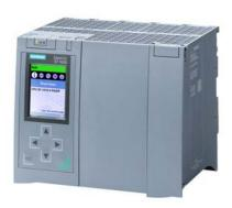
SIMATIC S7-1500, CPU 1518-4 PN/DP, central processing unit with 6 MB work memory for program and 60 MB for data, 1st interface: PROFINET IRT with 2-port switch, 2nd interface: PROFINET RT, 3rd interface: Ethernet, 4th interface: PROFIBUS, 1 ns bit-performance, SIMATIC Memory Card required
